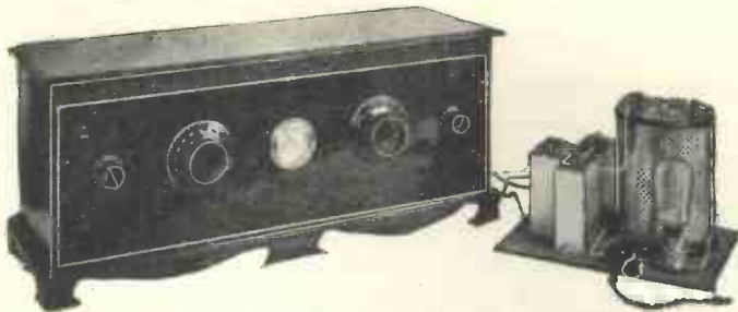
The rectifying unit on the right is added for A.C. working
