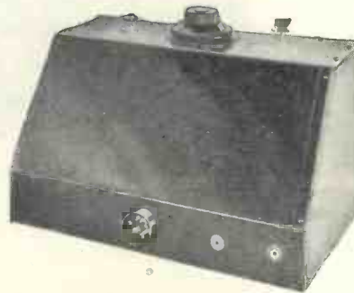
The controls at the top are the reaction condenser, main tuning control, and on-off switch. Below are the socket for the battery cord and the sockets for the frame aerial
