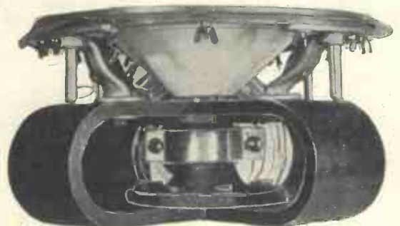
Plan view of the loud-speaker. Note the positions of the cone and magnets
