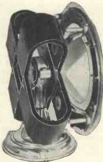
Side view of the loud-speaker showing size of permanent magnets
