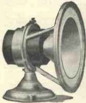
Although it is claimed to be cheaper than any other model on the market, the pot of the Epoch loud-speaker contains 7 lb. of No. 20-gauge enamelled wire and consumes .7 ampere at 6 volts. The makers are the Epoch Electrical Society, Ltd., of 53 Gracechurch Street, E.C.3
