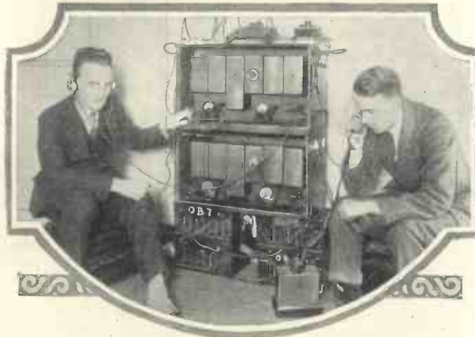
An "outside broadcast" amplifier such as might be used for relaying a play from a theatre
