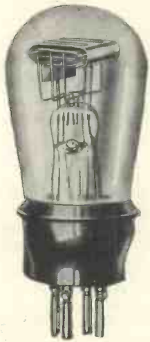
This is the HL210, made by Marconi and Osram. It is a most useful general-purpose valve, having an impedance of 25,000 ohms and an amplification of 15
