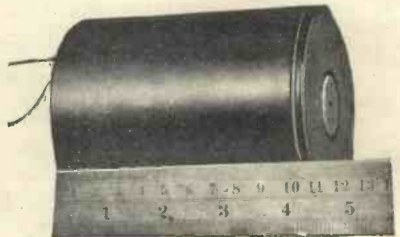
This photograph shows the small magnet "pot" of the front of the "Junior" Loud-speaker
