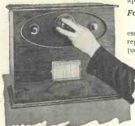
The dials from left to right are: anode-bend potentiometer, aerial condenser and reaction condenser
