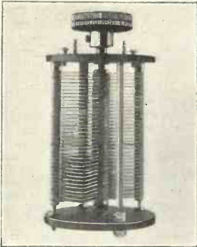
Although few condensers of this type are seen nowadays, they were in general use in the early days of broadcasting.
