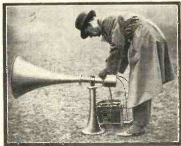
Connecting up a loud-speaker for public-address work.
