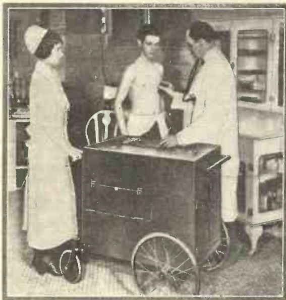
Portable Western Electric Stethophone in use.
