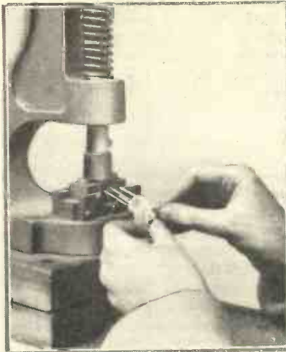
The electrode supports are cut the correct lengths.
