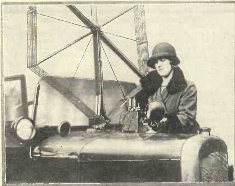
Small Car Equipped with Polar Twin Receiver.
