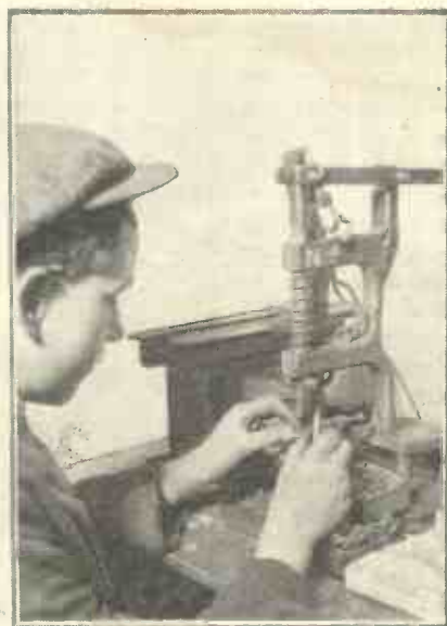
The stems are spot-welded to the electrodes.
