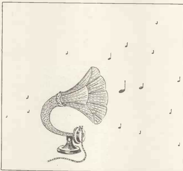
Fig. 3.—Relative Sizes of Notes Indicate Distribution of Sound from Horned Loud-speaker.
