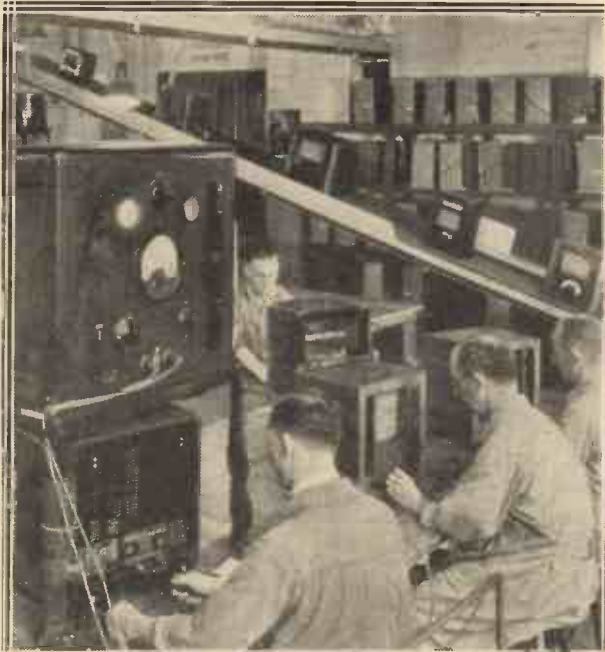
The manufacture of radio receivers in Germany has reached a very high standard of efficiency. Here is a corner of the Siemens factory where the complete sets undergo special high-tension voltage tests.
