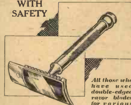
All those who have used double-edged razor blades for various cutting purposes will appreciate this suggestion for getting a better grip and control. The method also obviates the possibility of accident.
