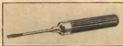
This screwdriver incorporates a "flash-lamp" in the handle which projects a spot of light on the work.
