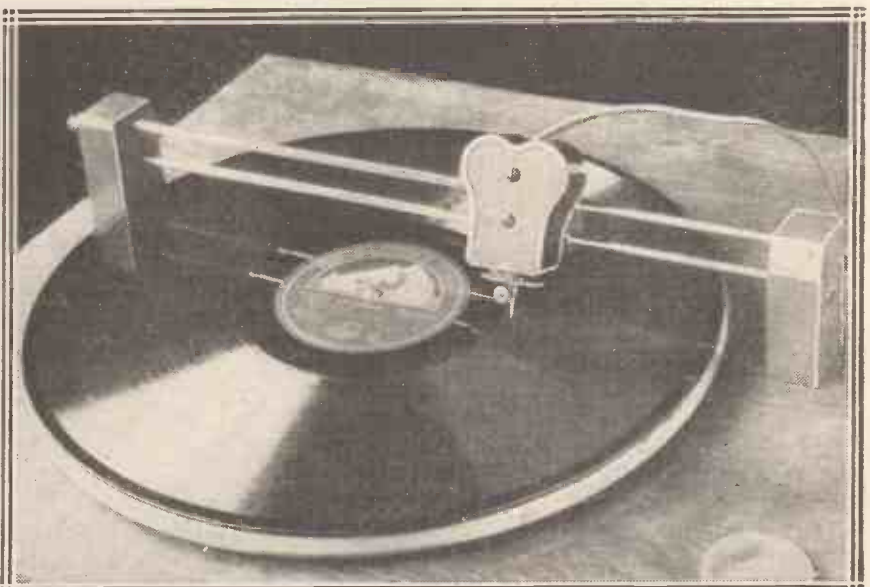
The pick-up moves straight across the record on two "rails," no swinging arm being employed. It is thus possible for the tracking to be exactly right both on the outmost and inmost tracks of the record.
