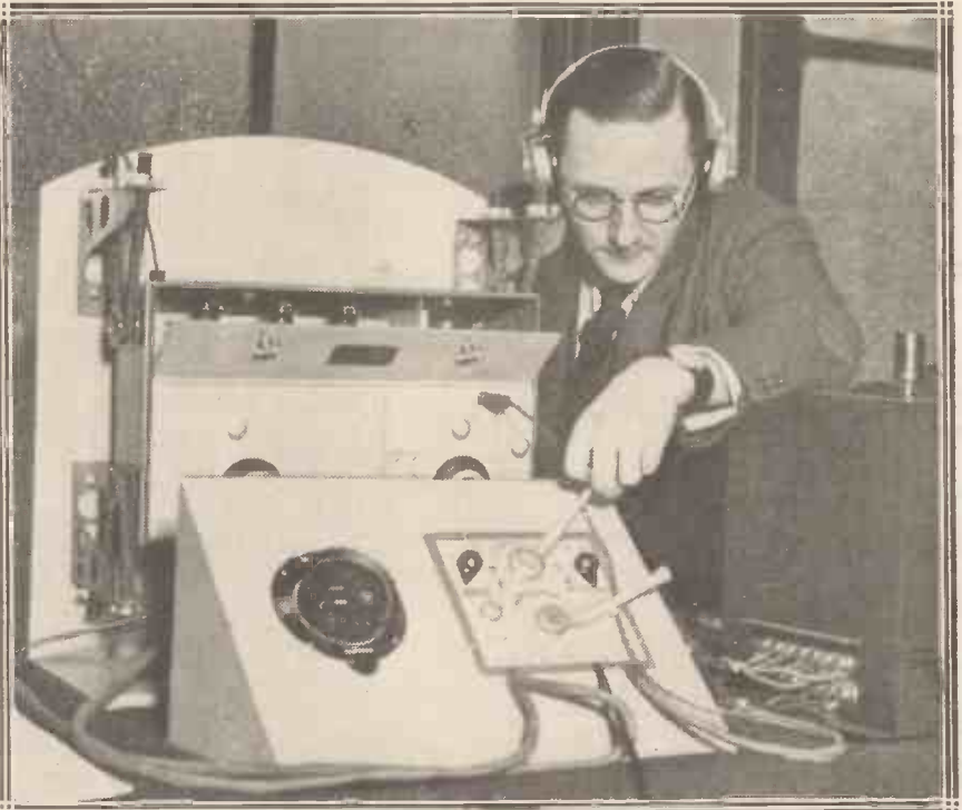
This ingenious radio apparatus helps the pilot flying a plane by a musical note, which alters in tone if he deviates from his radio-directed course.
