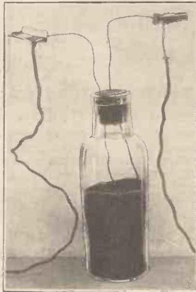
Two copper wires dip into a bottle containing soot. By raising or lowering one of these wires, resistance, and therefore volume, is varied.
