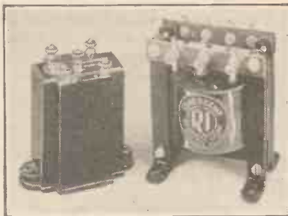
The R.I. quiescent push-pull input transformer and output choke. The primary inductance of the input transformer is 30 henries at zero D.C., and 20 henries with 1 milliamp. flowing.
