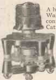
Differential Condenser. Slow-motion ratio approx. 9-1 is incorporated in the condenser and is controlled by the upper knob. direct drive being obtained on the lower knob. Cat. No. R/190. Capacity '0003 each half. Price 3/-.
