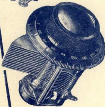
J.L.4 CONDENSER Slow-motion type (35/1). Capacity, ·0005. Complete with 3" dial, 7/6. Extra heavy gauge vanes. Rigid nickel-plated frame. High-grade ebonite insulation.
