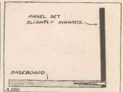
Fig. 4. The panel is "raked" slightly, and supported by the bracket shown in Fig. 3.
