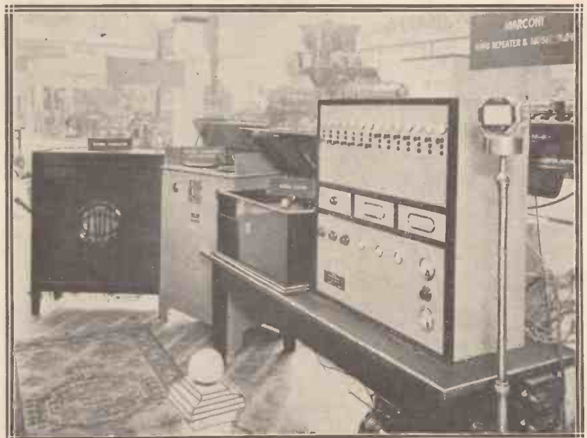
The gear illustrated above was used at the Shipping, Engineering and Machinery Exhibition at Olympia as a band repeater. It fed a large number of loud speakers installed throughout the hall, and was also employed to enable visitors, on the opening day, to hear the conversation which took place between the President of the Exhibition (Lord Wester Wemyss) and the Captains of the "Homeric" and "Empress of Britain."
