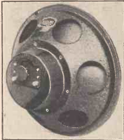
The Graham Farish cone loud-speaker chassis utilises a cone which is made of a fabric material. The suspension is remarkably free.
