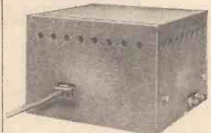
The Osram "All Power" Unit enables the Osram "Four" to be converted to "all mains" with the minimum amount of trouble. Five-pin valve-holders are already incorporated in the set.
