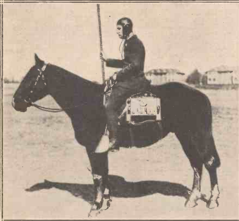
Radio for cavalrymen is the latest stunt in the U.S.A. The wireless set can be seen fixed to the saddle, while the horseman carries the aerial wound round his lance. It is claimed that by this means greater effectiveness in manoeuvres is obtained.
