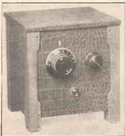
The "Eelex" short-wave adaptor is designed for use with broadcast receivers having one or more H.F. stages. It immediately converts the set into a short-wave super-heterodyne.
