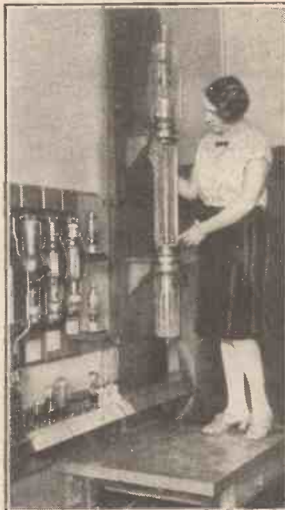
Here you see one of the huge transmitting valves referred to in this article, and which are for use in the KDKA broadcasting station.
