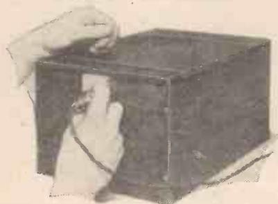
A safety device incorporated in a "Wireless Constructor" mains unit design. You cannot open the lid without first of all withdrawing the plug which connects the unit to the mains.
