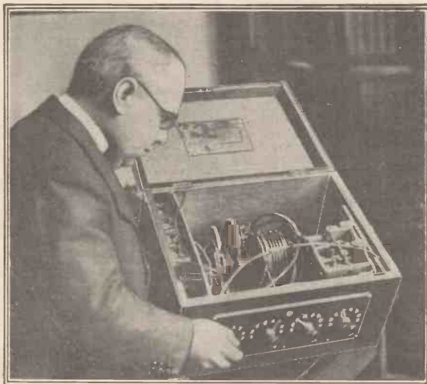
Pirates have been very active of late in the China seas, so this invention of Mr. Richardson, of York, should have real uses. It is a bullet-proof S.O.S. sender. It continues to give the S.O.S. signal and the ship's position by radio even when under fire.
