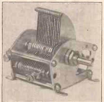
The Polar "Universal" condenser has a loose spindle and is constructed so as to enable two or more units to be "ganged" together without difficulty. This component is very sturdily made.
