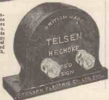
Telsen H.F. Chokes, designed to cover the whole wave-band range from 18 to 4,000 metres, extremely low self-capacity. Shrouded in Genuine Bakelite. Inductance 150,000 microhenries, resistance 400 ohms. Price 12/6 each.
