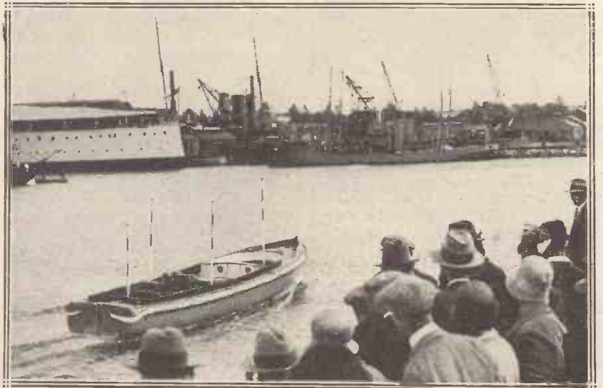
Visitors to the Portsmouth Navy Week show watching the performance of a motorboat which was entirely controlled by radio. It was a 35 ft. boat, and had not been demonstrated to the public before.
