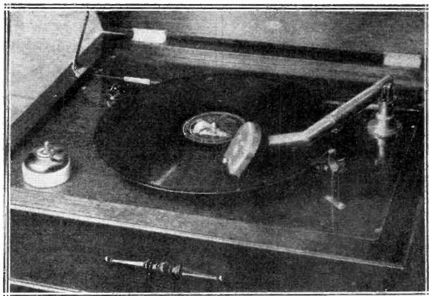
The turntable, on-off switch, and B.T.H. pick-up which form the top section of the electric gramophone.
