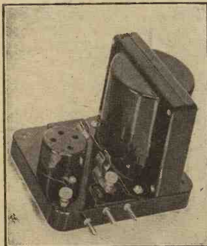
The Ediswan "Threesome" comprises an assembly of compact units. Above is the L.F. transformer unit.
