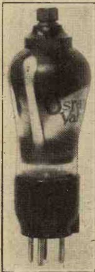
A modern screened-grid valve which is capable of tremendous amplification due to the high magnification factor. Owing to the peculiar construction it cannot be directly compared with the ordinary three-electrode valve, though the slope is below unity.
