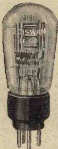
A 6-volt L.F. valve which has a slope of 1.5, its impedance being 10,000 ohms and the magnification factor 15. The curve of the valve is shown in column 3, whence it will be seen that although the magnification (variation of plate current for variation of grid volts) is high the valve will carry only a moderate grid swing, so obviously would be unsuitable for heavy inputs.
