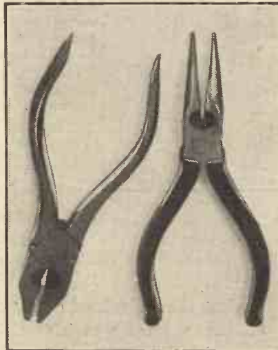
Two tools which set-makers find invaluable. (Left) A pair of flat-nosed cutting pliers, and (right) round-nosed cutting pliers. The latter are very useful for wiring a set.
