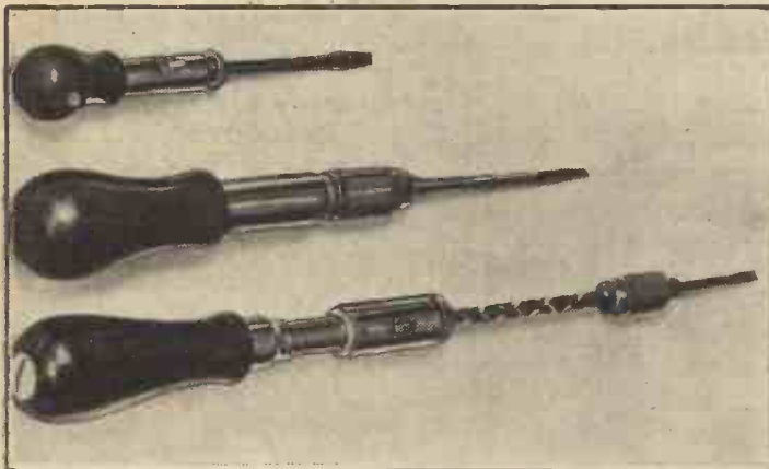
Ratchet and Archimedean screwdrivers enable screws to be driven home very quickly and easily.
