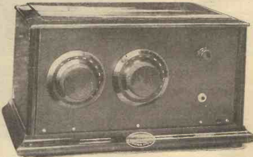
Two tuning dials and a reaction dial figure on the symmetrically arranged panel. There is also a telephone receiver plug which operates as an on-off switch in addition to its normal duty.
