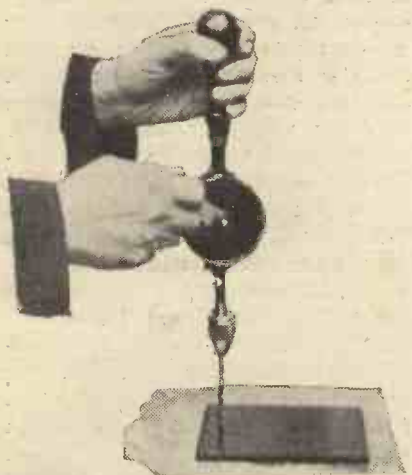
The panel should be laid on a piece of paper or cloth, and the drill held perfectly straight.
