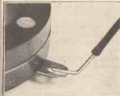
The completed connection, after cleaning with duster.
