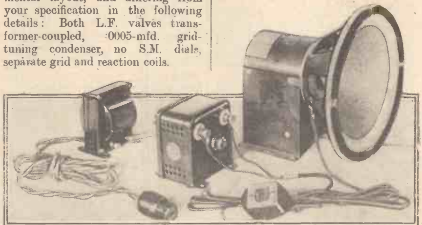
One interesting use for a rectifying unit is to provide current for a moving-coil loud speaker from A.C. mains, as shown above.
