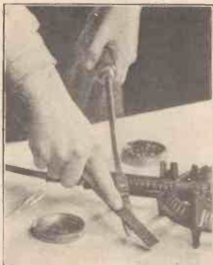
The iron should be carefully kept clean and free from oxide deposits.
