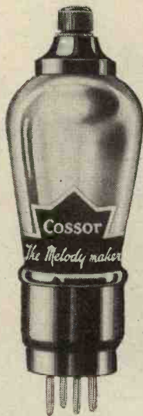
This is the new type of Cossor screened-grid H.F. valve, which among other makes is available for various voltages. Note the difference in design between this valve and that of a year ago shown in the heading of this article. The horizontal type of screened-grid valve is now being replaced by the upright 4-pin and cap type such as is shown here. The horizontal Marconi & Osram S.625 will be still available and is not being taken off the market.
