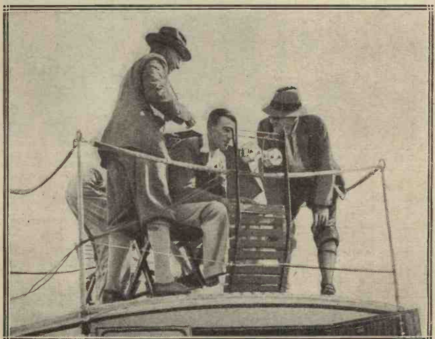
Here is the latest broadcasting van in use. It contains all the amplifiers necessary for outside broadcasts while on top is a platform from which events can be viewed and their descriptions broadcast in moderate comfort.
