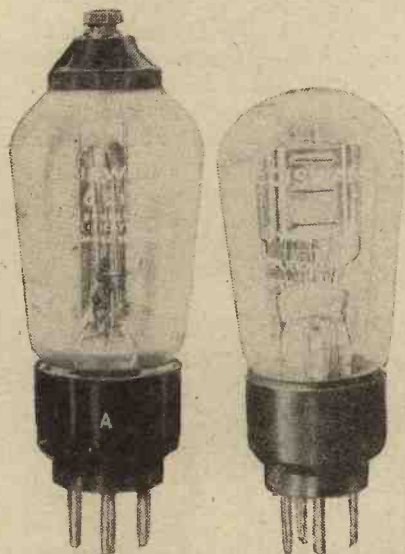
The Edison screened grid two-volter, (left), and the P.V. 610 6-volt power valve.
