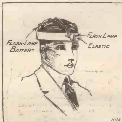
The "headlight" in position, showing the method of fixing and wiring.
