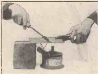
Soldering on to metal screens is not an easy task unless the metal is perfectly clean and is reasonably hot.
