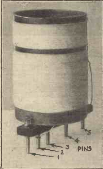
The coil used for the reception of the ordinary broadcast wave-lengths. Note the spacing of the pins; the numbers are referred to in the text.
