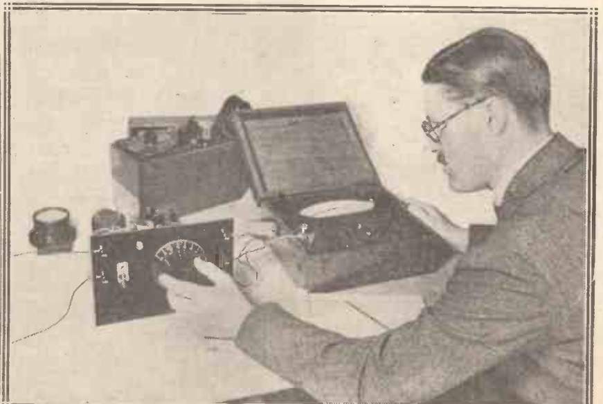
Testing the strength of 5 GB by means of a microammeter and a sensitive crystal set.
