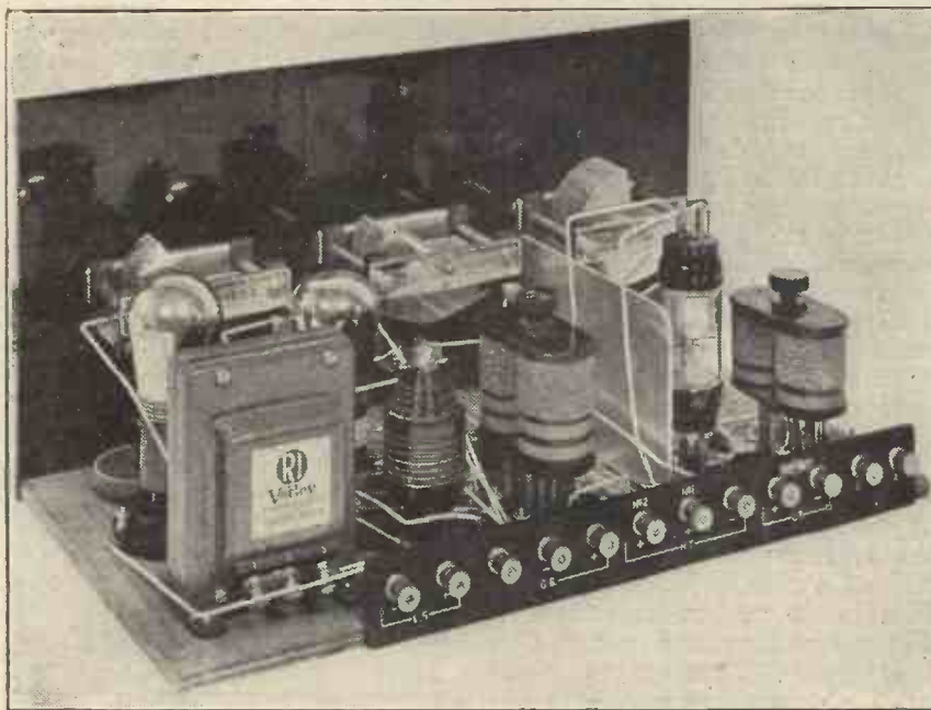
Binocular coils were employed to cut down magnetic coupling.
