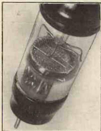
A "close-up" of the electrodes of the shielded valve.
