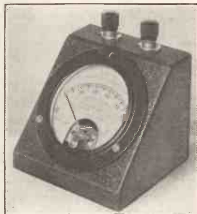
The H.F. Thermo Galvanometer (Weston Electrical Inst. Co.).
