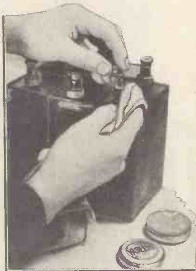
An Accumulator Hint: Terminals should be cleaned and coated with a little vaseline or petroleum jelly to avoid corrosion.
