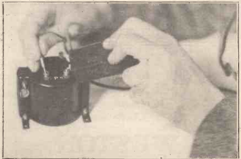
Testing a transformer with a battery and phones in series.
