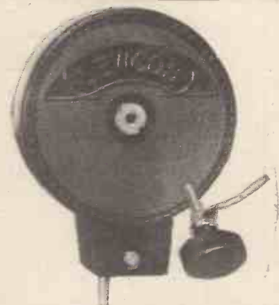
A novel centre-tapped coil ("Lewocos").
