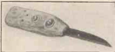
A handy keyhole saw, made from an old hacksaw blade.
