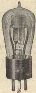
A typical rectifying valve, as used for A.C. rectification.
