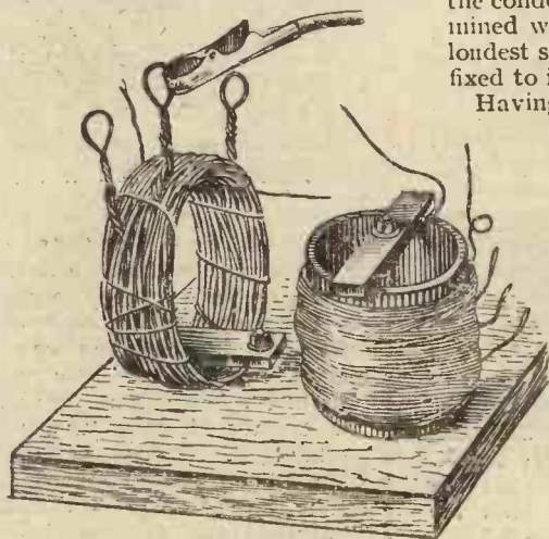
Fig. 3. This sketch shows how the tapped coils are made.
