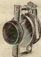
IGRANIC Filament Rheostat, 30 ohm type Designed for controlling all types of Dull Emitter Valves. It is smoothly and evenly variable over its whole resistance range and affords very fine selectivity. Suitable for controlling up to four valves according to the type of valve used. Current carrying capacity 0.4 amp. Price, with screws and drilling template for panel mounting 7/-
