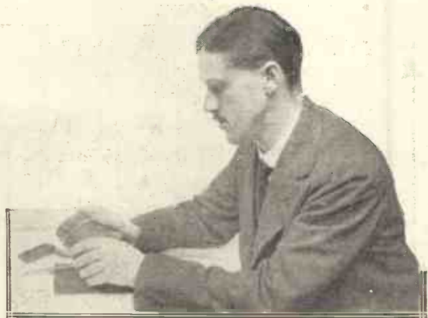
How to wind the coil. Keep the turns close to one another with the thumb, and wind tightly.
