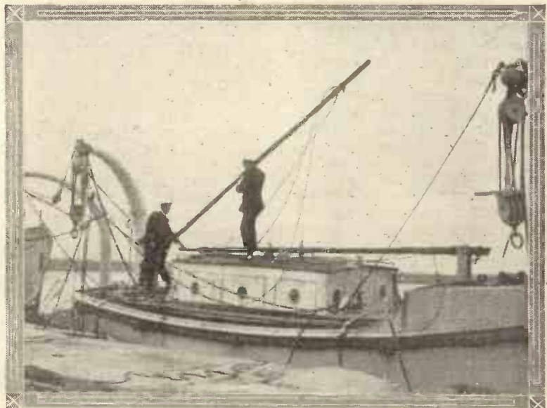
The aerial mast on a lifeboat of the s.s. "Aquitania" fitted with wireless.
