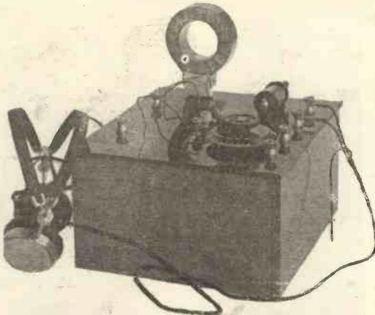
When it is desired to hear Chelmsford, the shorting plug is withdrawn, and a number 150 coil inserted.
