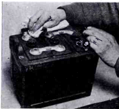
Removing collected dust and copper sulphate from the top of your batteries insures a longer life for the battery and less noise in your receiver
