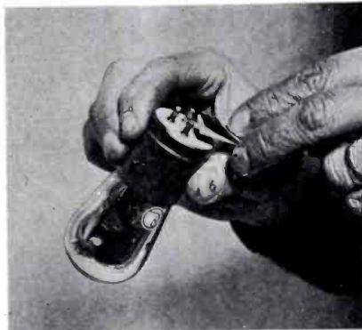
The application of a fine file or emery paper to the tube contacts makes for better contact and a quieter set
