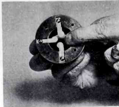
Bending up the tube socket contact prongs is good practice provided the prongs are made of elastic springy metal
