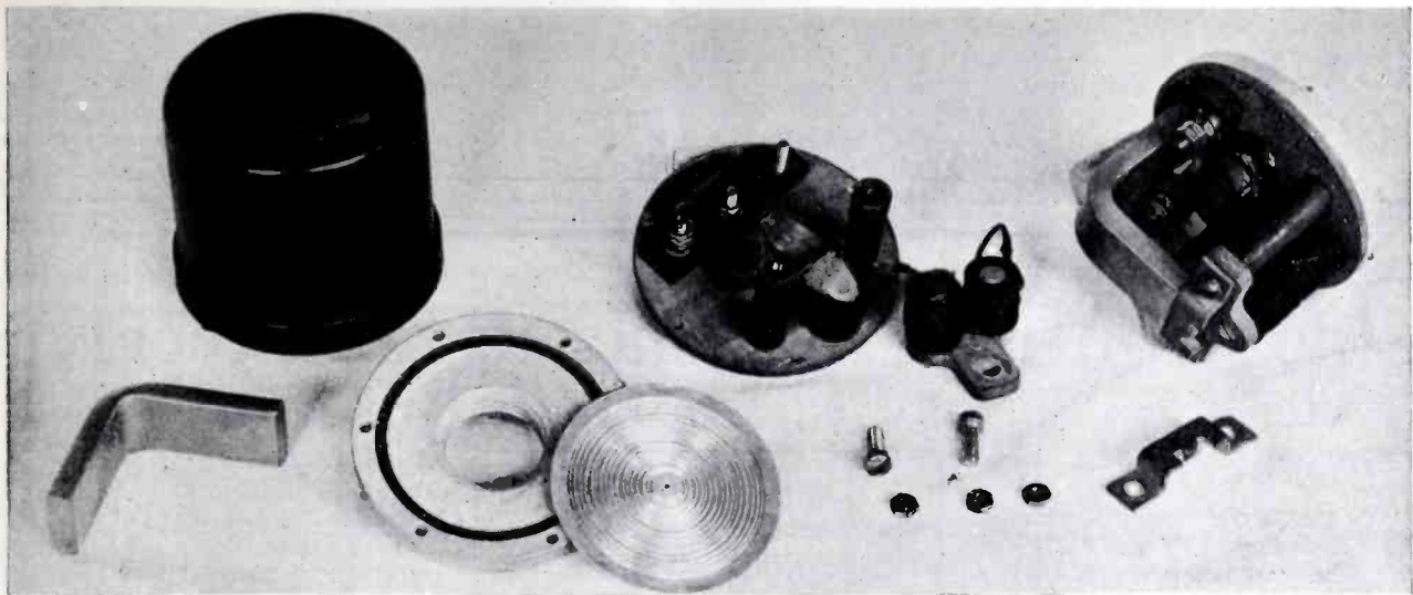
Figure 4—The ordinary balanced armature permanent magnet loud speaker unit
