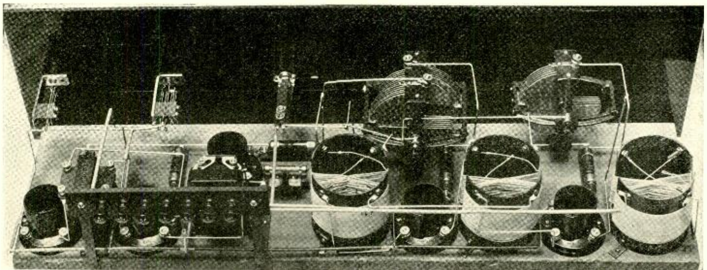
This tilted rear view of the D-coil shows the positions of the astatic transformers and tuning condensers
