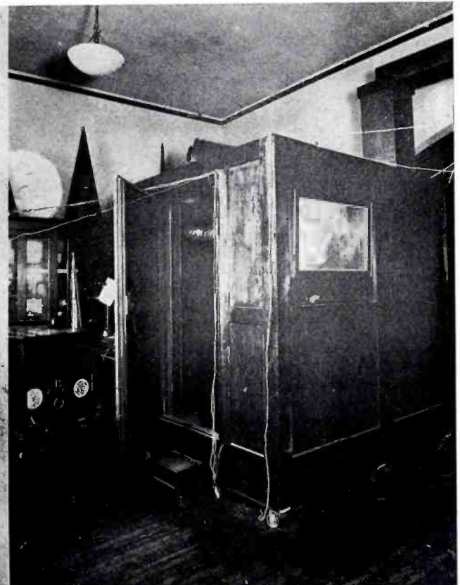
Exterior view of the portable sound proof booth built especially for acoustic experiments
