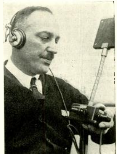
A. Pawelek, radio engineer of the S.S. Columbus, holding the latest type of apparatus for testing spark gap of wireless transmitting set. Its construction is similar to a miniature crystal radio set. Antenna is enclosed in wood block with crystal detector and headphone plug in base
