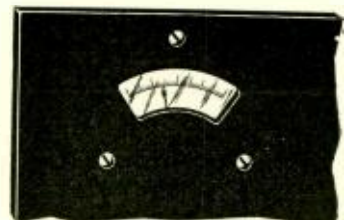
Meter mounted behind the panel
