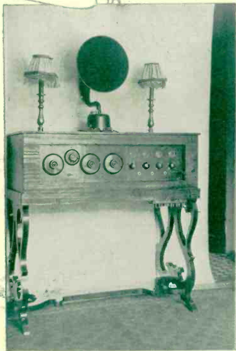
J. B. Michaels of Bristol, Conn., encloses his set in a case of Japanese driftwood; batteries and chargers too; phone connection block at right provides for six headsets. The panel and dials are of mahogany
