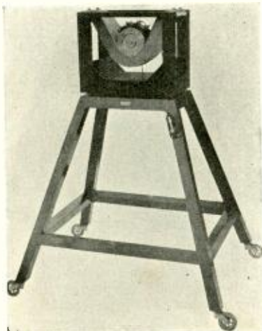
The Marconi microphone used in British broadcasting stations. With this instrument it is possible to speak in a natural voice more than 30 feet away and get perfect transmission
