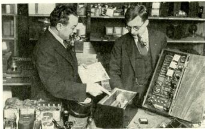
Mr. Dubilier (left), radio manufacturer, and Harry W. Houck (right), radio inventor, with the original and the perfected models of the super-ducon, the new device which is designed to replace the batteries used in the operation of radio receivers
