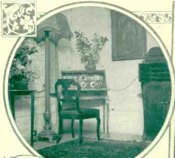
Austin H. Martin of Glen Ellyn, Ill., places home-made receiver in discarded desk with batteries in drawer, and uses Victrola for loud speaker
