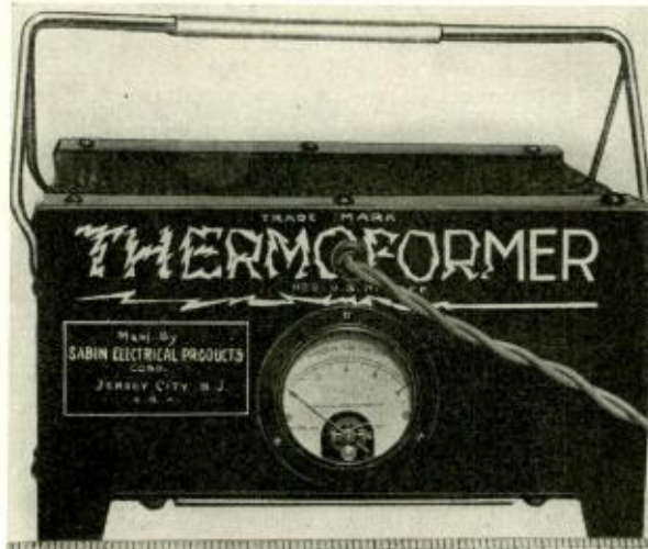
The Thermoformer that makes possible the operation of tubes on A. C. or D. C. lighting circuits
