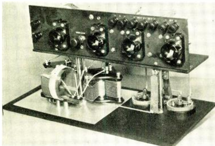
Figure 1—The portable receiver assembled. Showing the tube panel and the reverse of the front panel on which one of the R. F. pickle-bottle transformers is mounted
