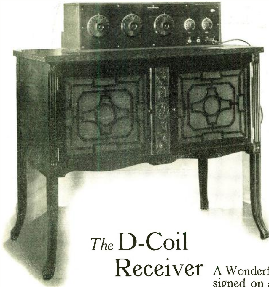
The D-Coil receiver is seen resting on the top of a console victrola. The output of the receiver is connected to a phonograph attachment which is attached to the victrola. The panel of the receiver is mahogany colored and all the dials are of the same color. The cabinet has a veneer of dark brown leather over the wood and since the victrola is mahogany, the whole setting blends in very nicely
