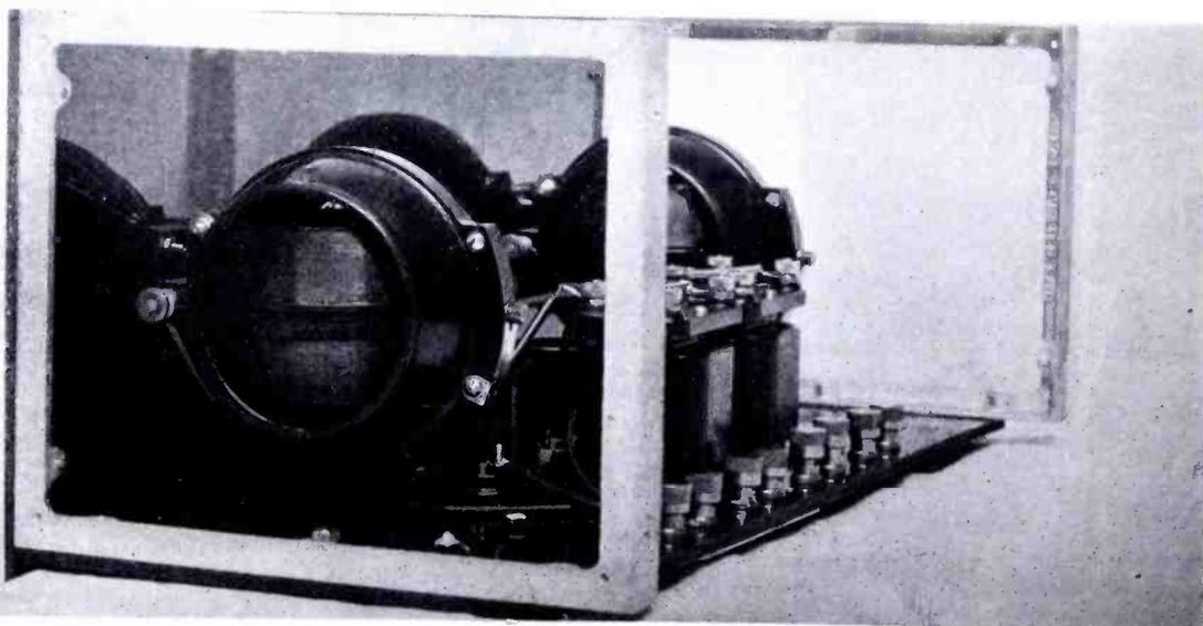
The simplicity of the receiver is evident in this end view. Note how cast aluminum frames are used to support the front and sub-panels
