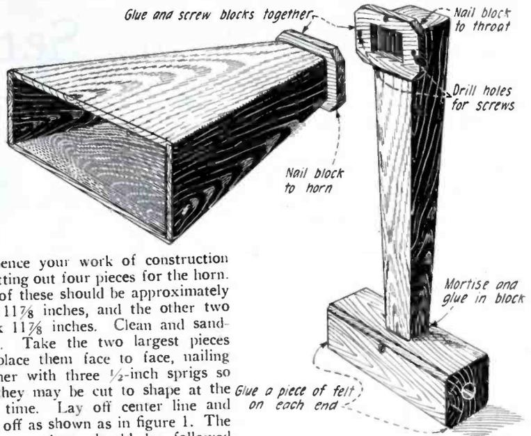
about  $1\frac{1}{2}$  inches apart. Glue one edge and nail large piece to sides of smaller ones. Then nail other side on, turn over and nail bottom of horn to sides. If not quite square, a little pressure on the corners will true it. Nail the throat the same way, but before nailing cut  $1\frac{3}{4}$  inches off as shown in figure 3 to allow for block.
