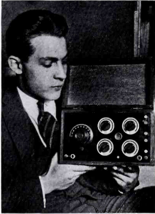
A miniature five-tube radio frequency, detector and audio frequency set using UV-199 tubes built by Sidney Kasindorf of New York and exhibited at the recent N. Y. radio show
