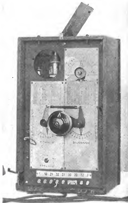
The tuning unit with front removed. The plug and socket on the left and right is provided so that the instrument can be tuned approximately to any wavelength depending upon the dimensions of the aerial. The knob in the center provides limited tuning and operates two circuits simultaneously. The knob in the top right hand corner varies the extent of reaction within fixed limits. In one position it produces maximum telephony signals and when the reaction coupling is increased it is suitable for rendering C.W. telegraphy audible
