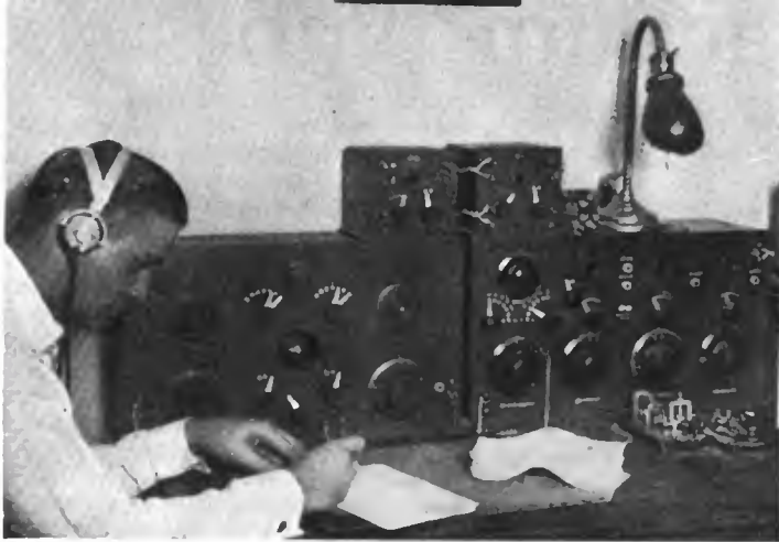
A complex, regenerative receiver, with three tuned circuits, employing variometers, extensively used by experienced amateurs. This type of receiver is more difficult to operate than those of the single-circuit type. It is highly selective and very efficient
