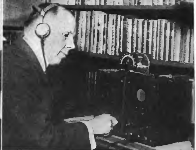
Another type of single-circuit regenerative broadcast receiver which is extensively used by the radio public. It has a vacuum tube detector and two steps of audio frequency amplification, making it possible to operate a loud speaker, if desired
