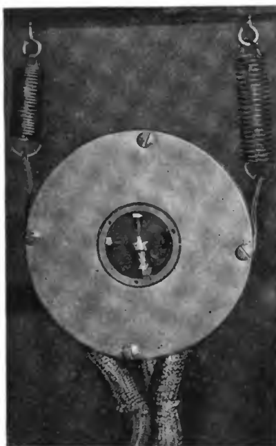
The New Thomas Glow-Discharge Transmitter showing position of electrodes
