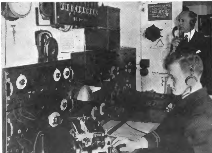
In the radio room of the "America," showing the operator, and in the background, J. Horace Porter, Marine Manager of the Radio Corporation of America, using the ship-to-shore radio telephone. Conventional telephone instruments in any part of the ship may be connected into the new system.
