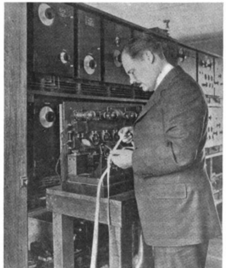
Dr. Goldsmith's high speed ink recorder in operation at Riverhead with E. W. F. Alexanderson examining tape
