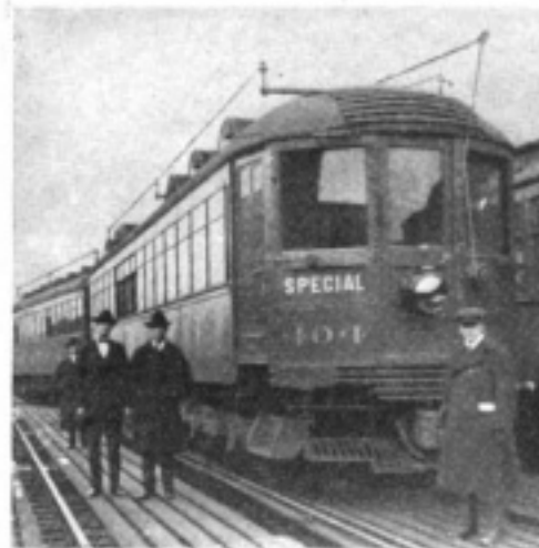
Chicago is continuing its experiments with radio receiving equipment for its elevated trains, using an antenna strung above the cars
