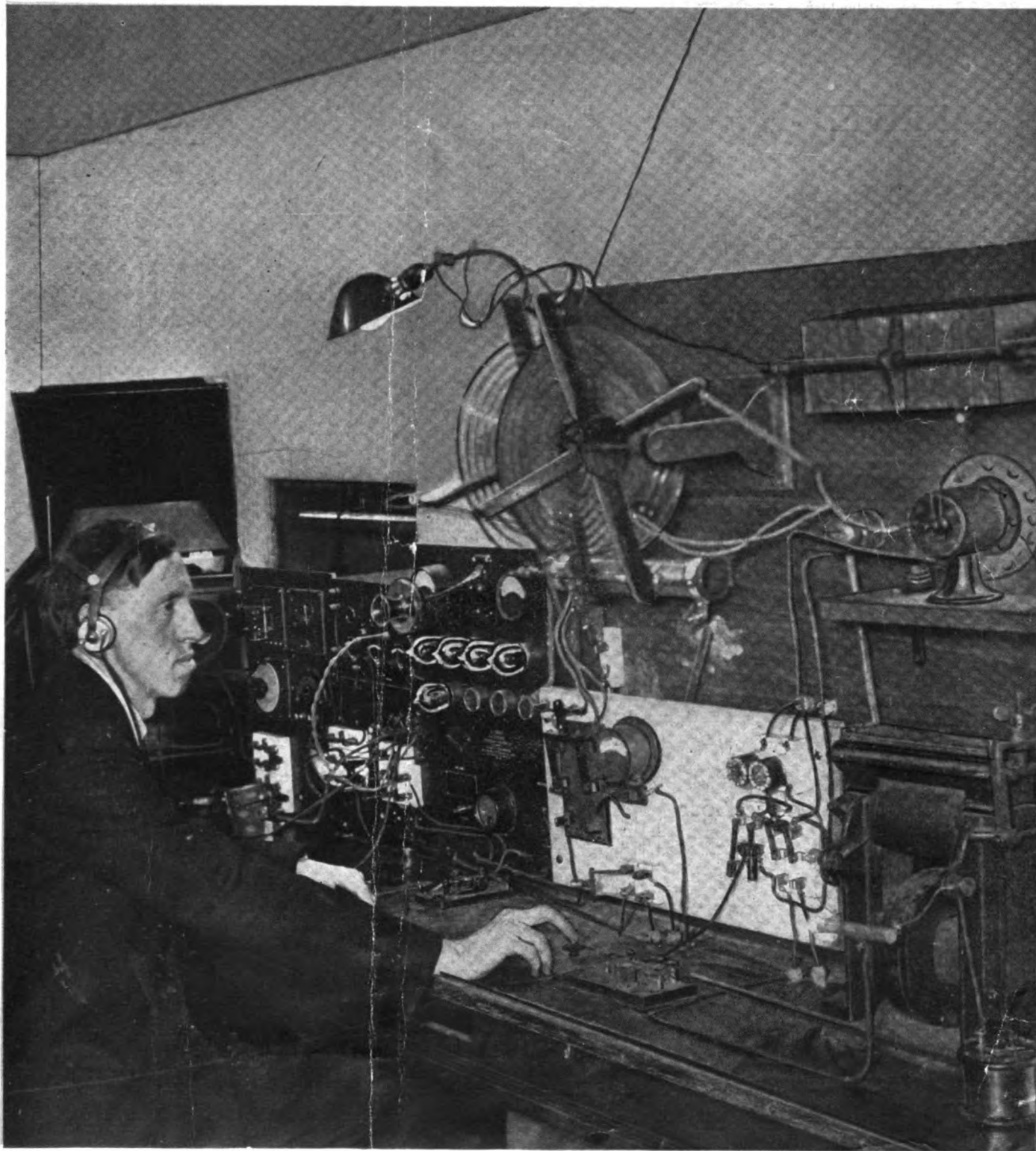
Prof. J. C. Jensen at key of radio station of the Nebraska Wesleyan University comprising rotary and quenched spark equipment and eight-tube radiophone
