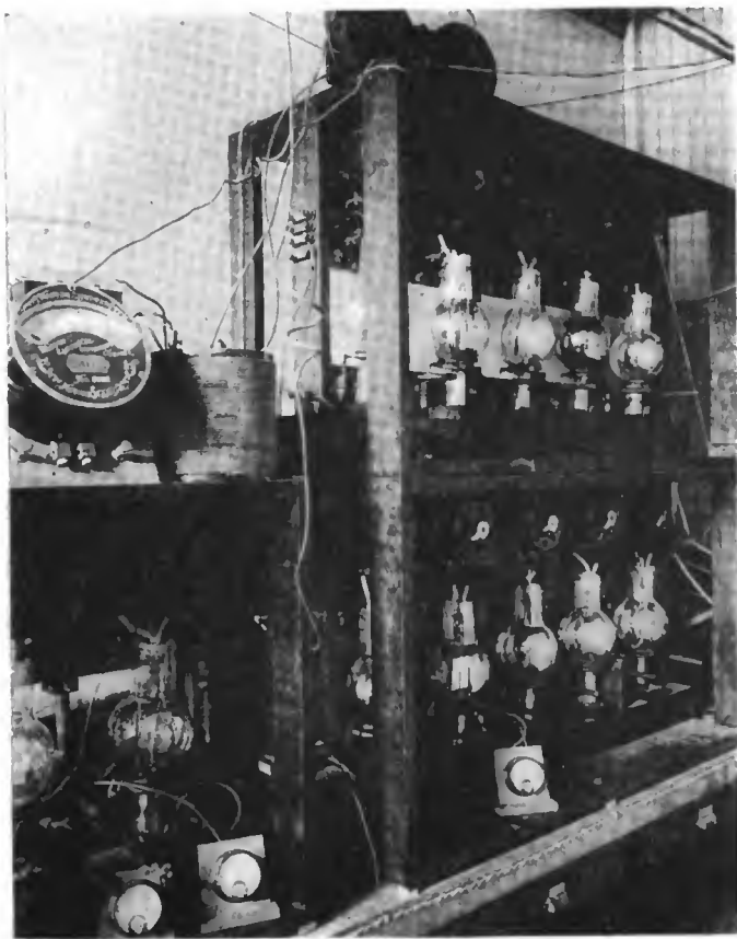
Dr. Goldsmith's radiophone set, showing the dozen vacuum tubes which were used to generate several horsepower for wireless telephony regularly conducted over a distance of 160 miles
