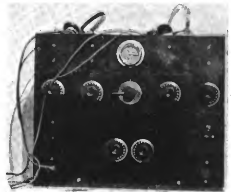
Figure 1—Complete Set Top row (left to right)—Grid leaks with condensers. Fixed condensers. Clock. Small coil. Grid leaks without condensers. Second row—Five variable condensers. Two .005. Two .008. One .00175. On left of tuning coils—22.5-45 volt batteries. Two jacks for phones. On right of tuning coils—Rheostat. Vacuum tube.
