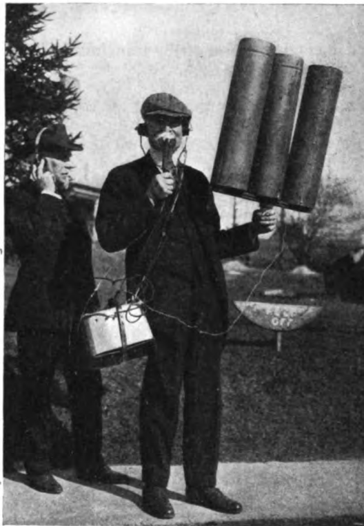
W. W. MacFarlane of Philadelphia with his radio-telephone that establishes fifty-yard communication by stovepipe aerial
