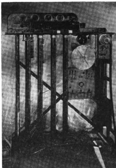
Photographic device for printing wireless messages on tape with a speed of 400 words a minute
