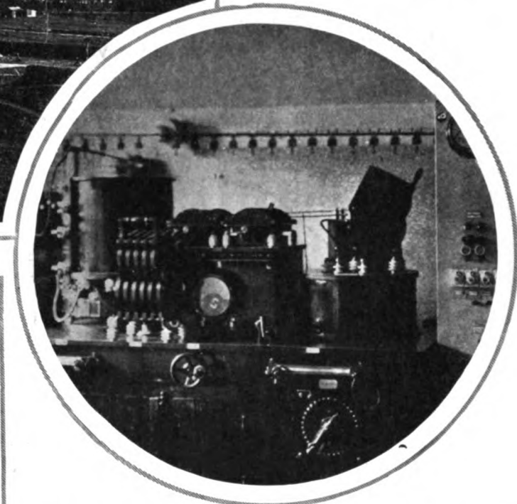
Above, in circle, the transmitting apparatus which was hooked up to the antenna on the 85-meter tower shown in the upper view
