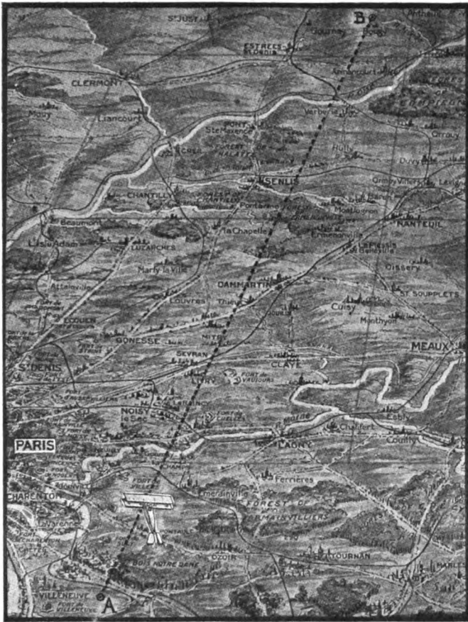
Figure 106—How an airplane must be steered off the direct course to allow for side wind drift
