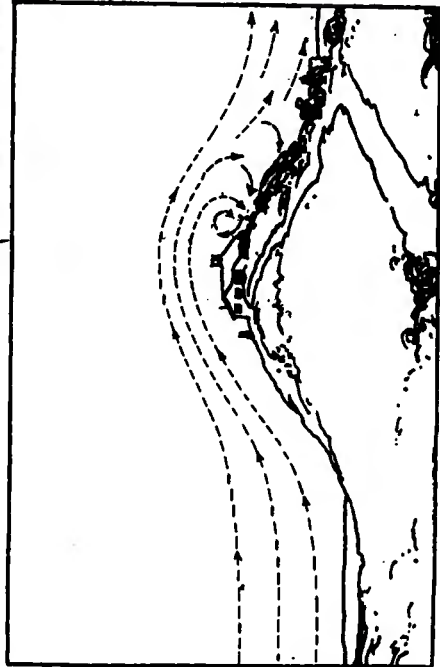
Figure 84 (Upper)—Action of the surface cataract Figure 86 (Lower)—Eddies, or bumps, in lee of obstacles
