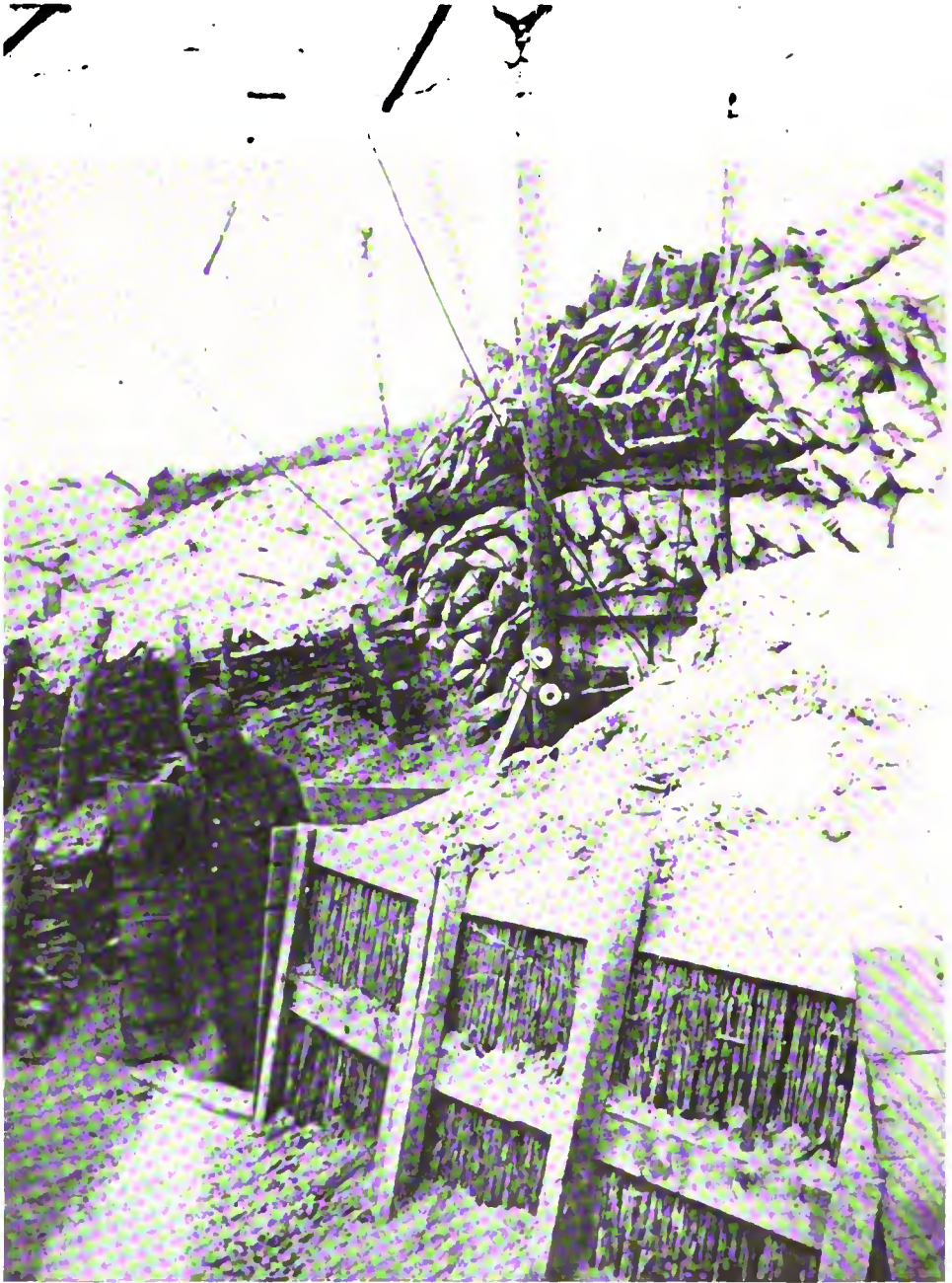
This view of a French wireless equipment in the second line of trenches is representative of the conditions awaiting American wireless men. The photograph clearly indicates the use of horizontal aerials suspended by pulleys for quick lowering. It is also worthy of note that the antenna is suspended but a few feet above the natural surface of the ground
