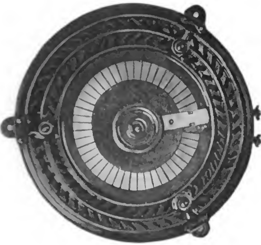
Figure 57.—Showing the general appearance of the Cutler Hammer type of field rheostat for regulating the field current of a dynamo or motor. The rheostat is made up of composition resistance wire baked in a heat-proof insulating cement and mounted in a metal case. The wire is tapped at intervals and leads are attached to brass studs over which a sliding contact moves
